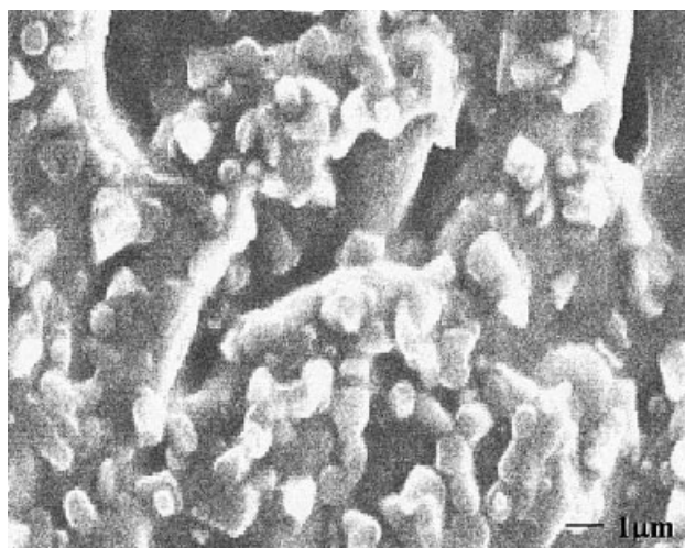
Figure 4 SEM micrographs of vacuum-evaporated PPV-ether films with a thickness of >2000 Å.
